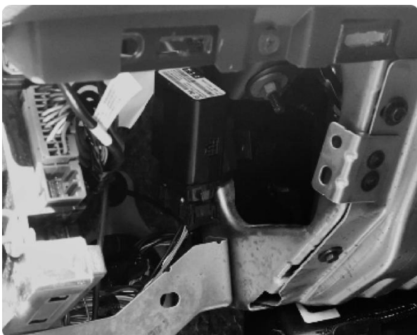
FT1 mounted under dash using OBDII Y cable & tie straps to securely fasten device to chassis of vehicle
