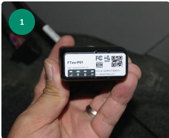
Connect the device to your OBD Y cable, this assumes the OBD Y male end is connected to the Diagnostic port of the vehicle. Look for a Red LED as an indicator of power.
