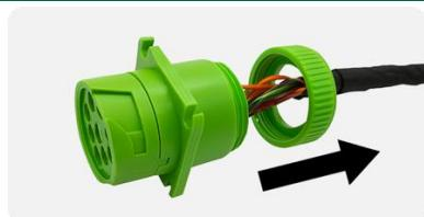
Step 2 Grip the wires at the back of the cartridge and remove the core connector and adapter together. Ensure that you do not damage or move the terminals inside. This will make re-insertion into the core connector easier.
