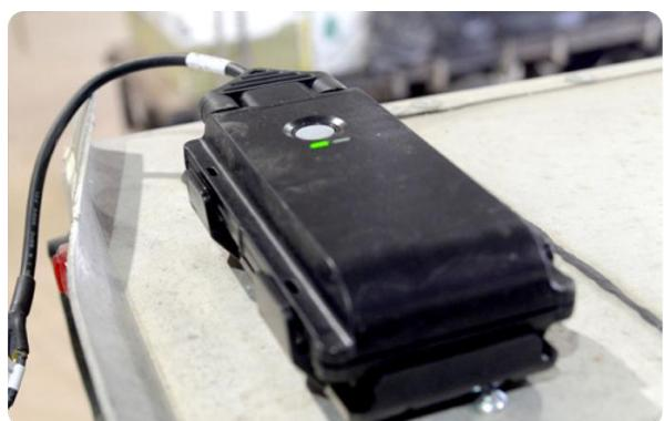
**3.** Mount the unit in the cradle. Make sure the tamper switch is pressed.
