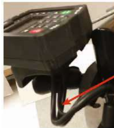
Ball joint to the side to allow for strain-free cable routing.
